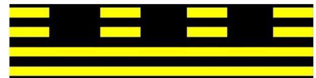
Fig 2. Runway Hold Position Marking
