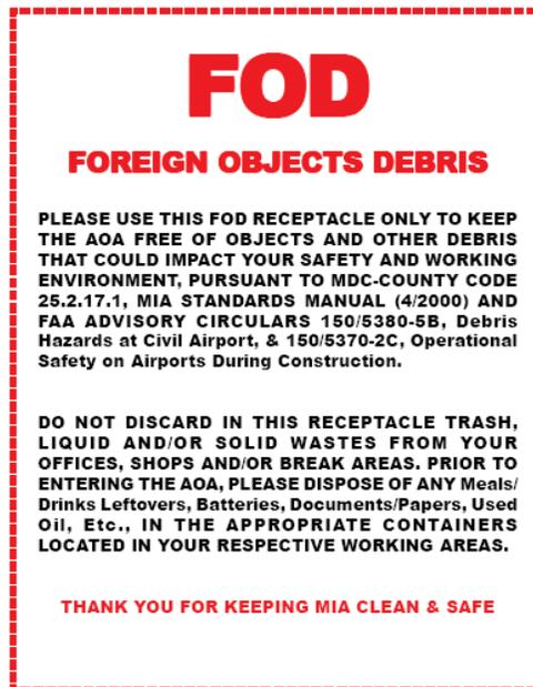
Figure 60. Foreign Objects Debris (FOD) label
