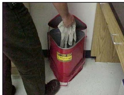
Figure 39. Disposal of oil rags in labeled containers
